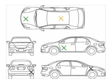
Cosmetic Panel / paint = Green Minor Scratches / Dents = Grey Damaged / Dented = Black Previous Body Repairs = Orange Rust = Red
